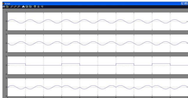
Figure 6.(1)carrier signal(2) 180° phase shift carrier(3) modulating signal(4) modulated signal
